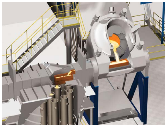
Figure 1 Cutaway of a production 1.4 \times 10^4 kg VIM furnace (reproduced by permission of ALD Vacuum Technologies).
