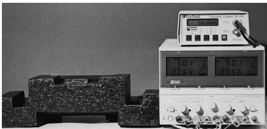
Fig. 2. Magnetic detector (on the left) with power pack and frequency meter.
